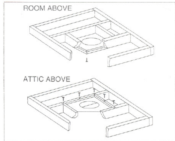
Figure 13 Installing the firestop spacer
